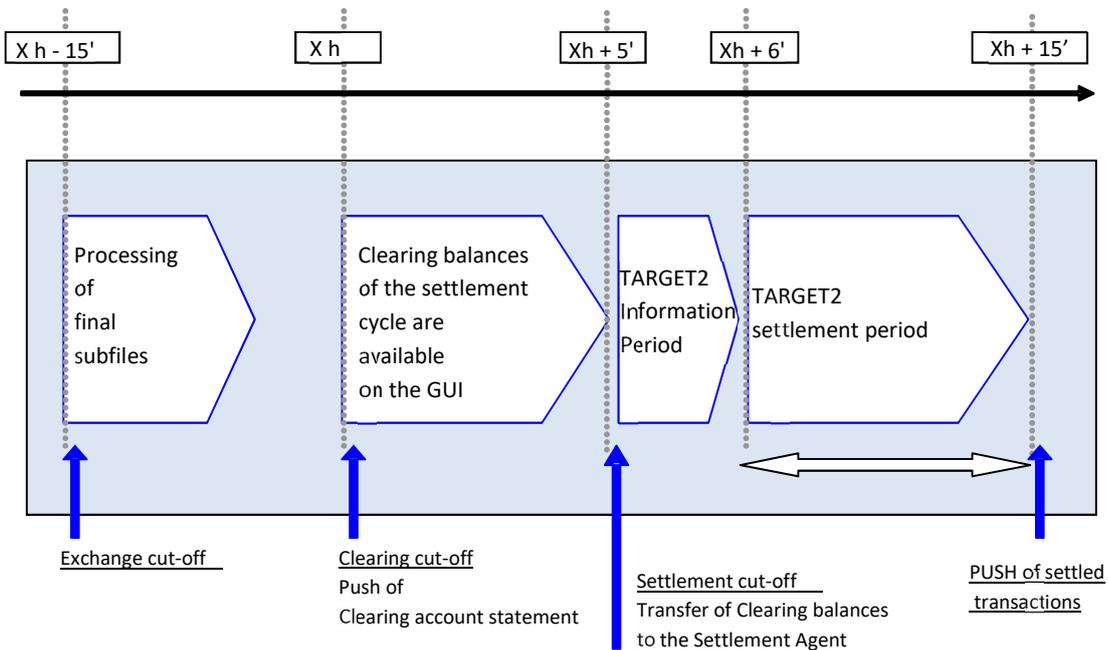
The following chart illustrates the Clearing and settlement cycle applicable to Transactions sent on D and settled on D+N (SDD Core and B2B services):
